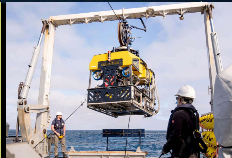
Remotely operated vehicle (ROV) SuBastian waits for deployment from RV Falkor at Flinders Reef in the Coral Sea. It has a suite of sensors and scientific sampling equipment, and can dive to 4,500 metres.
